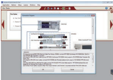
Push-Button Automation for PCIe 4.0 Base Spec Rx Testing with the Anritsu MP1800A BERT
